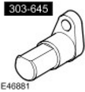
Crankshaft locking tool 303-645
