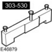
Camshaft setting/locking tool 303-530
